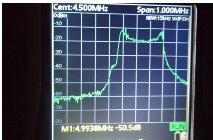
Fig. 25 Bandwidth occupied with 2128 Hz modulation applied (100 KHz/div)
