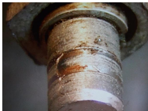
Figs 6,7 and 8 Score mark and hollow-point grub screw
