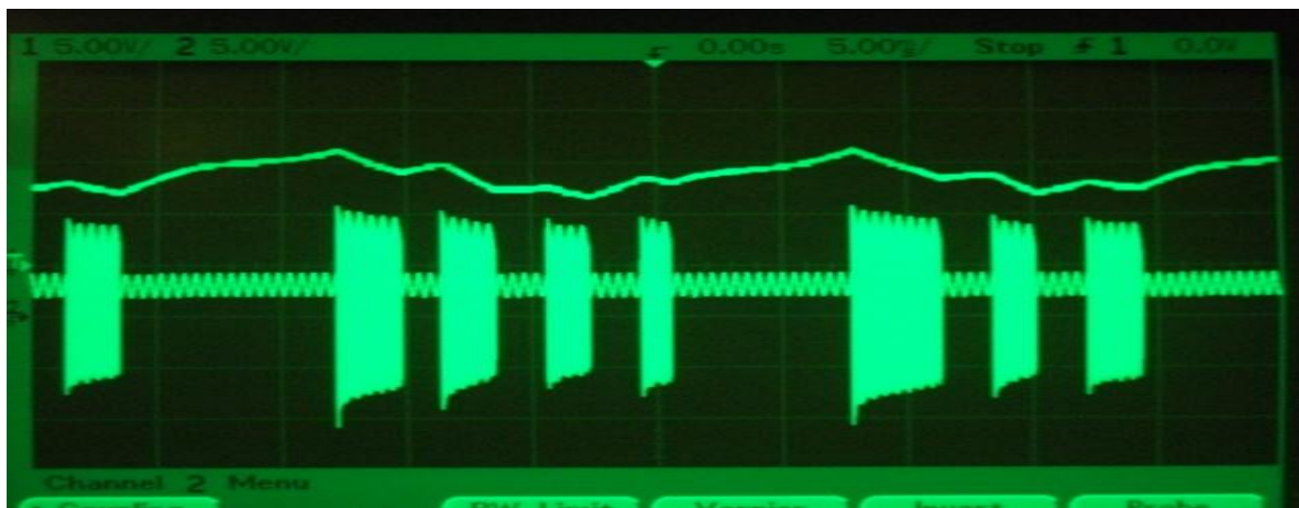
Fig. 21 Maximum setting of 2128 modulation, missing cycles of 2128 Hz
