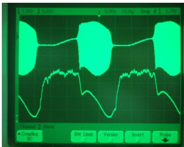
Fig. 27 Modulation frequency, 21.28 KHz. Horizontal scale 10 \mu s/div.
