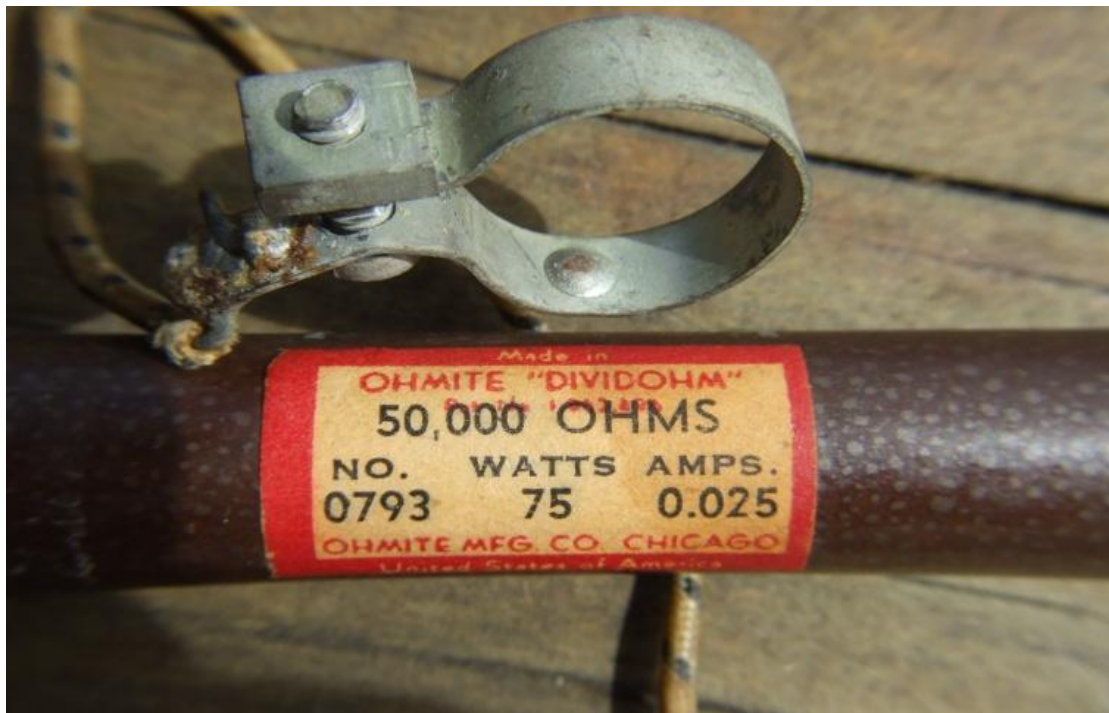
Figs 11 and 12 50 K preset, clamp contact and severed winding
