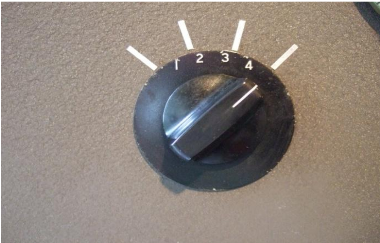
Fig. 5 Frequency range switch, white strips added to show the true positions
