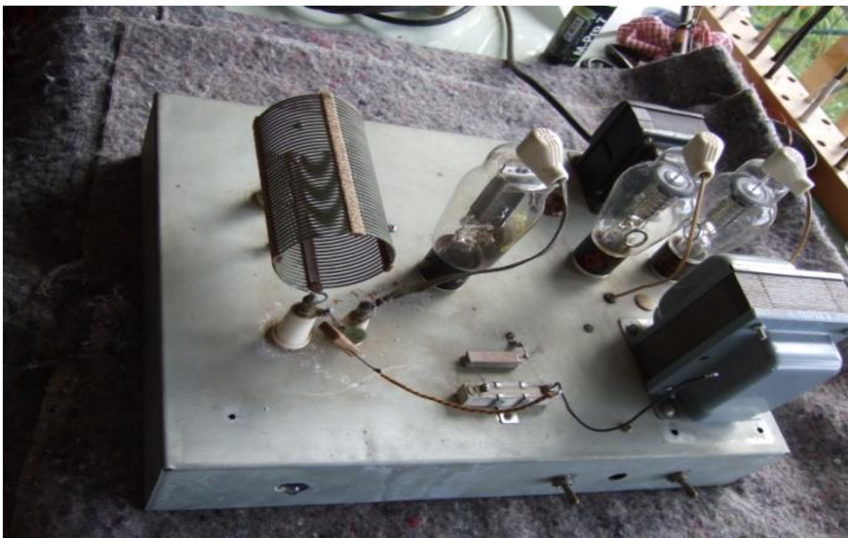
Fig. 9 RF oscillator and PSU (Faulty preset replaced by 1K2 and 1K0 in series)
