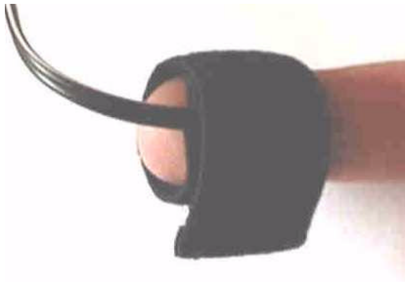
Figure 5. Positioning of finger sensor
