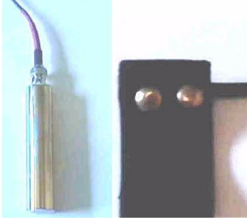
Figure 4. F-scan hand held electrode (left) and finger sensor (right)
