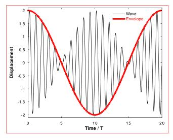
i.e. the beat frequency = the difference in frequency between the two sources.
