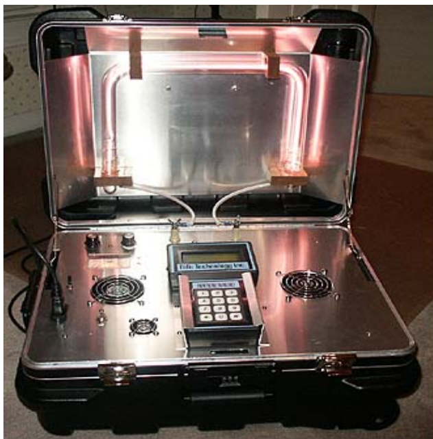
300 Watt PEP pulsed field transmitter. 27.125 MHz carrier frequency. Pulse rate capability 225 KHz.
