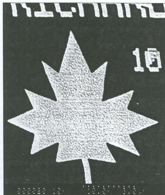
Fig. 9. Scanning electron micrograph of the same area as Fig. 8 except that it was made using the Robinson backscatter detector at the higher voltage. The details of the points, outer edges and internal angles of the maple leaf are clearly shown although this mode of operation introduces some distortion to the image.
