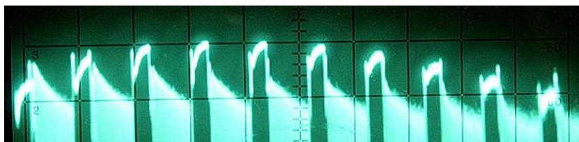
Spectrograph of 5000 Hz transmitted wave from a Rife/Bare Device at 50% Duty Cycle.
